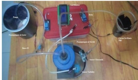
**Gambar 5.** Hasil Rancangan Sistem Monitoring Kedalaman Dan Kekeruhan Air
