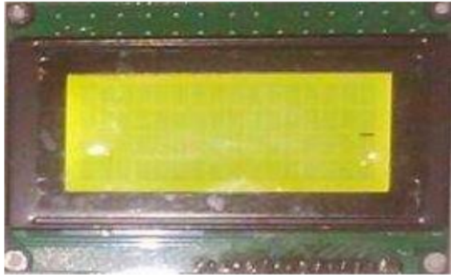
Gambar 2. Liquid Crystal Display (LCD)20x4
