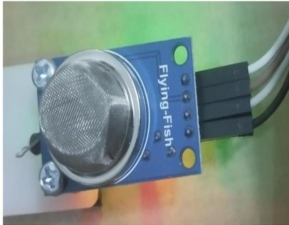
**Gambar 7. Pengujian Sensor CO<sub>2</sub> MQ-135**
