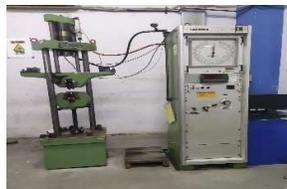
**Gambar 5** Mesin Uji Tarik di Laboratorium POLINEMA
