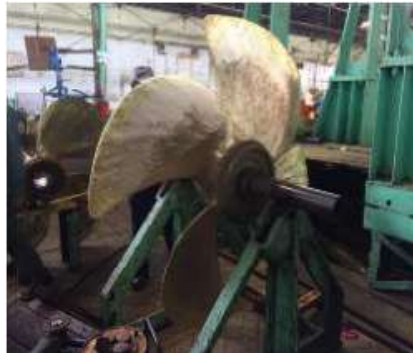
Gambar 6. Proses Balancing Propeller
