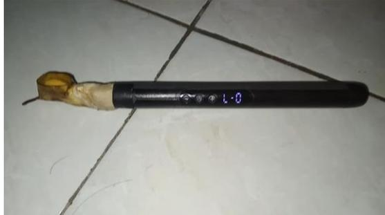
**Gambar 3 Canting eletirk portable ketika keadaan low batery**
